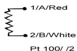
Typical connections for 2,3 & 4 wire Resistance Thermometers
