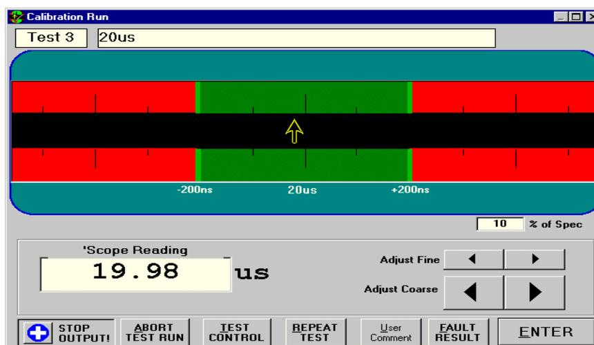
This example is of a period calibration test, but the display for amplitude is similar. Use the **Adjust Fine** and **Adjust Coarse** buttons to vary the value shown in the 'Scope Reading' box until it matches the reading of the oscilloscope.
