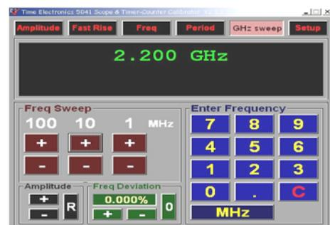
For direct read-out of error, a deviation feature is provided - this allows the frequency to be deviated up to +/-10% with a 0.001% resolution. Please note that the deviation setting is limited by the frequency setting resolution of 25KHz. This means that it is not always possible to achieve the deviation accuracy shown in the display. Deviation control is only usable above 15MHz.
