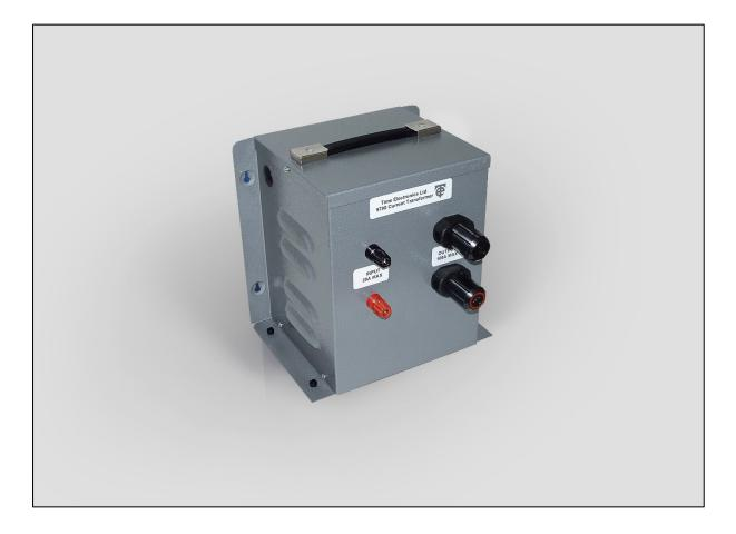
The 9790 is a heavy-duty current transformer mounted in a steel case. It is suitable for use with Time Electronics 5025 and 5051 multifunction calibrators, as well as the 5077 power calibrator. It extends the AC current capability to 100 A RMS.
