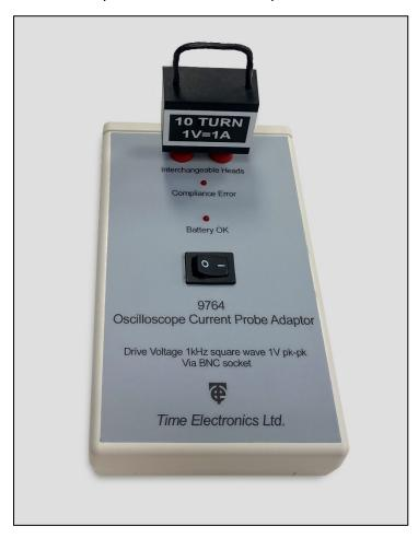
Then clamp the probe from the oscilloscope to the coil of the head to calibrate.
