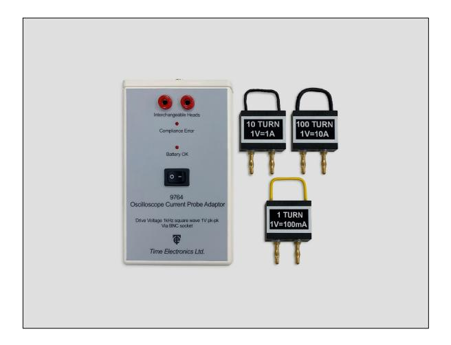
The 9764 current probe adaptor converts the amplitude output of an oscilloscope calibrator to a square-wave current in the wire loop of one of three interchangeable heads. The adaptor can be used with the 5045 scope calibrator, or 5025 / 5051 models with scope calibration options fitted.
