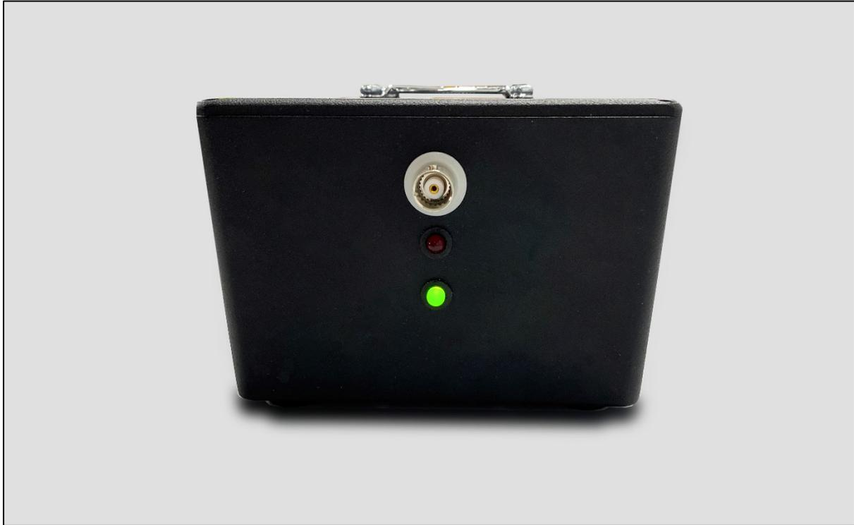
The 9762 is connected to the 5045 via the rear panel 10 MHz reference input.
