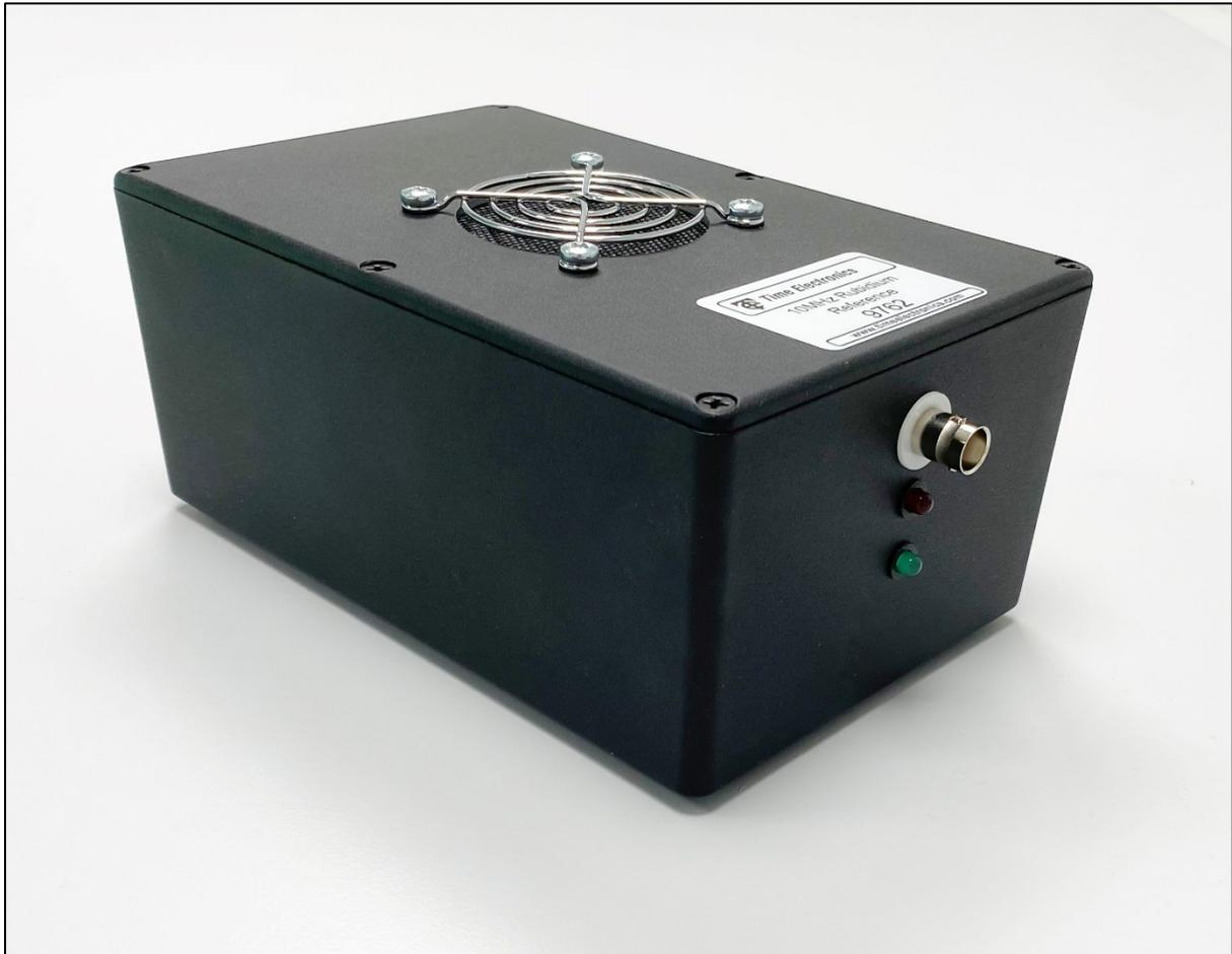
The 9762 is a high accuracy rubidium atomic frequency reference. It is designed to enhance the output frequency of the 5045 oscilloscope calibrator up to 10 MHz.
