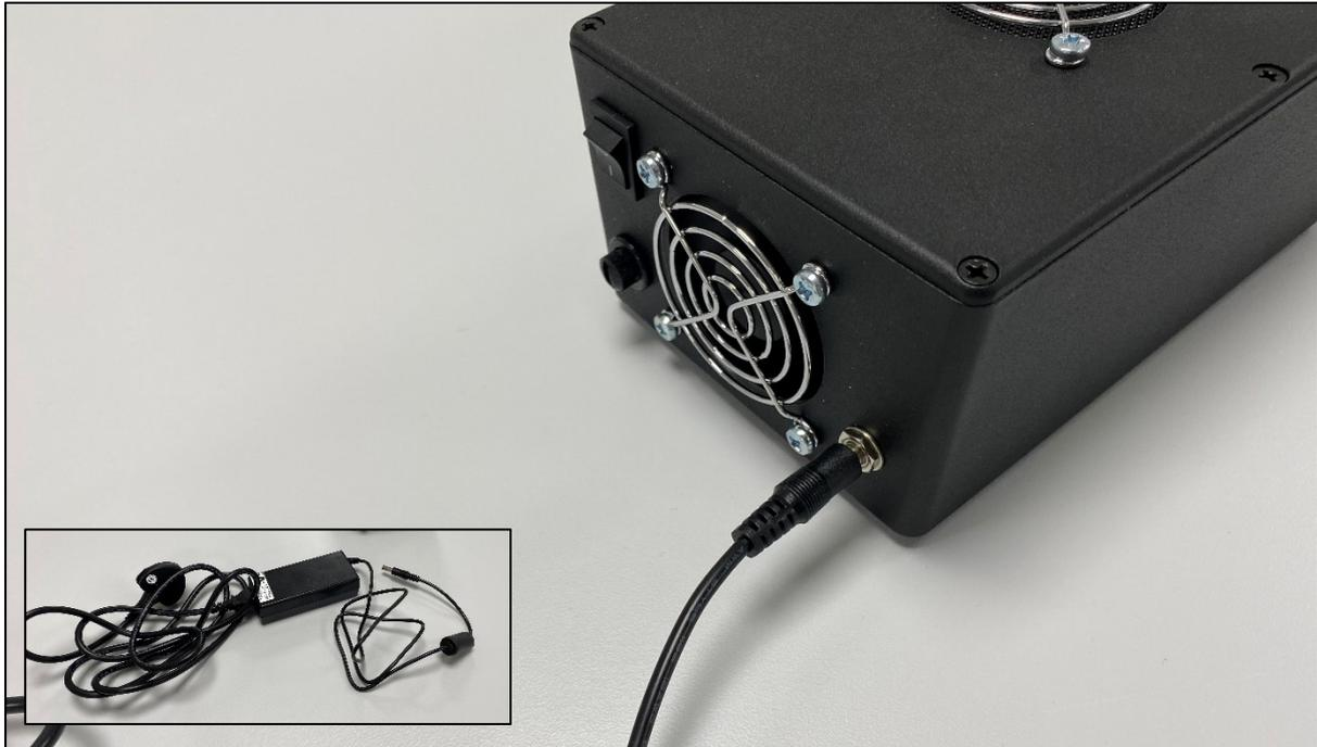
On the rear of the 9762 there is an on/off switch, 350mA fuse, external 24V DC power supply connection, and fan. Do not obstruct the fan.
