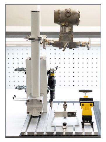
The angle bracket can also be used with the support clamp. Remove the u-bolt clamps and place the bracket in the support clamp. Tighten with the electric screwdriver.
