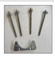
Remove the front and middle sections of the support clamp.
