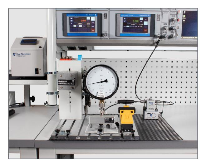
The 8030B is connected to the 7115 contamination trap (supplied separately), then to the 8100 manifold with the analogue gauge being tested.
