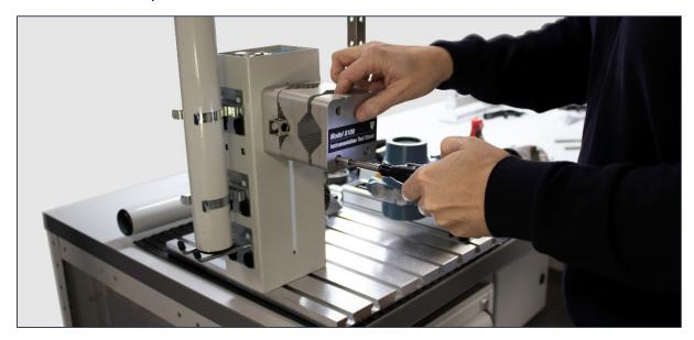
The **electric screwdriver** is a useful tool and speeds up the screwing and unscrewing of the cylinder bolts on the support clamp. It is also a practical solution for various other tasks.
