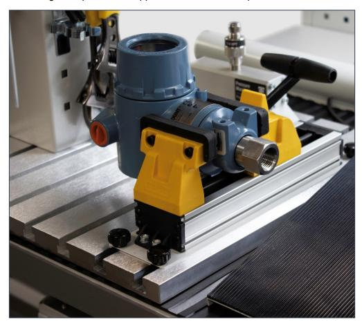
It can be re-positioned by loosening the thumb screws and sliding into the tracks.
