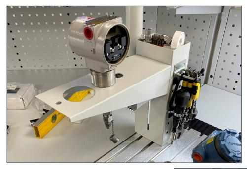
To do this, unscrew and remove the pole clamps.
