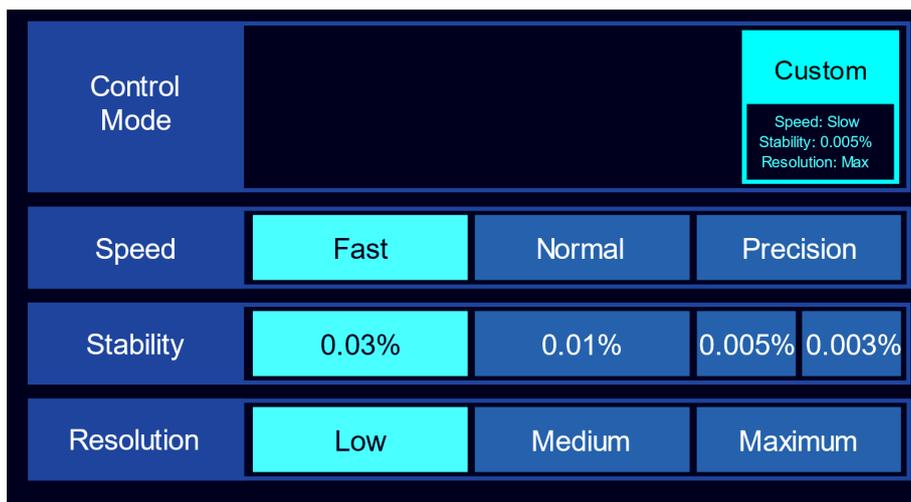
**Note:** In custom mode you can select precision at 0.003% stability. This mode requires a leak free set up with optimal working conditions for the controller to perform properly.
