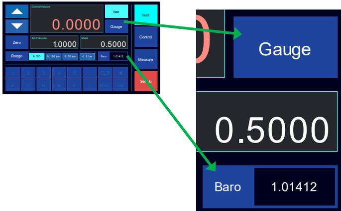
If the optional barometric sensor is fitted, a box labelled 'Baro' shows the current atmospheric pressure.
