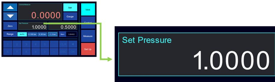
This value shows the set pressure that the controller will control to when in Control mode. The set pressure can be changed by pressing Set Pressure Box.
