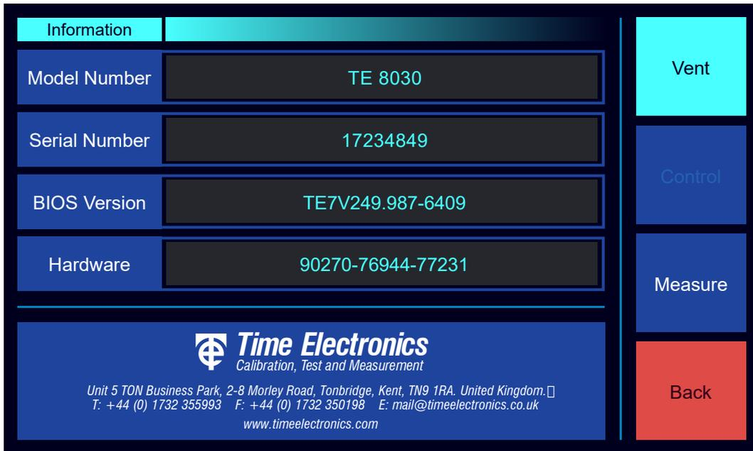
In the Information menu, it is possible to view the instrument Model number, Serial number, BIOS version and hardware number.
