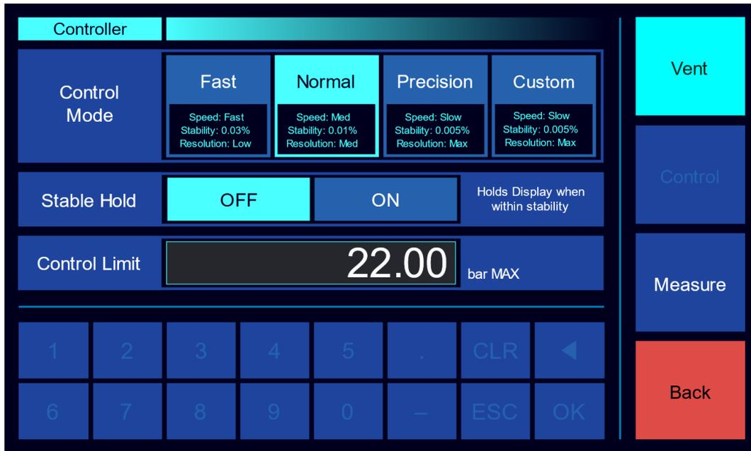
The Control Menu allows adjustment of the Control Mode, Supply Pressure and Control Limit. It also allows access to the custom control mode menu.
