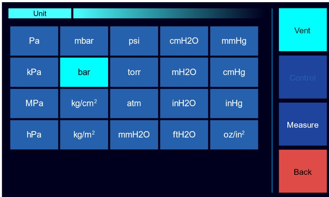
In the Unit menu, it is possible to change to instrument to a different pressure unit. This menu is also available from the main control screen as shown earlier.
