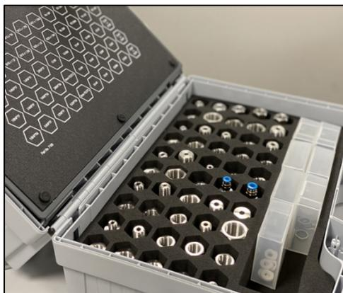
The 7198 pressure adaptor kit can also be used to make connections from the 7115 to various UUTs with different thread types.
