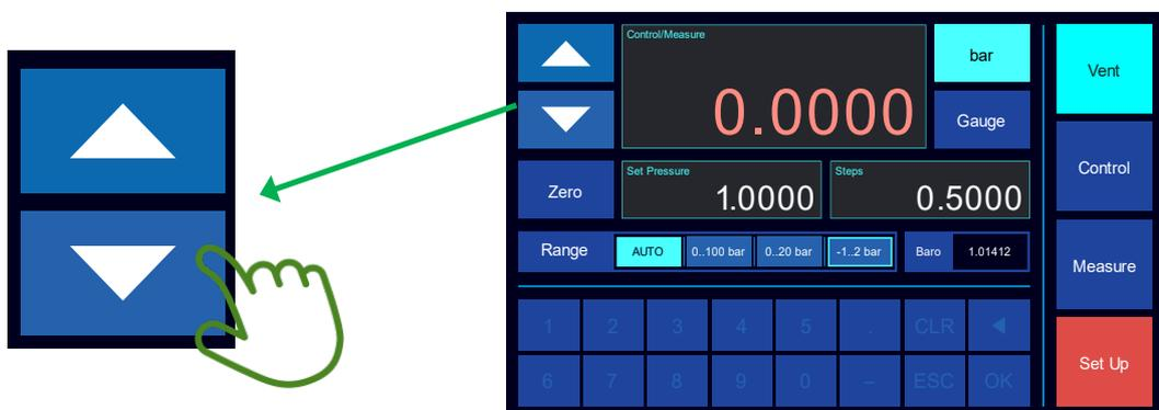
By touching on the up or down button the set pressure will be increased or decreased by the step value. This feature is very useful to control up or down between specific test points, for example cardinal points on an analogue gauge.
