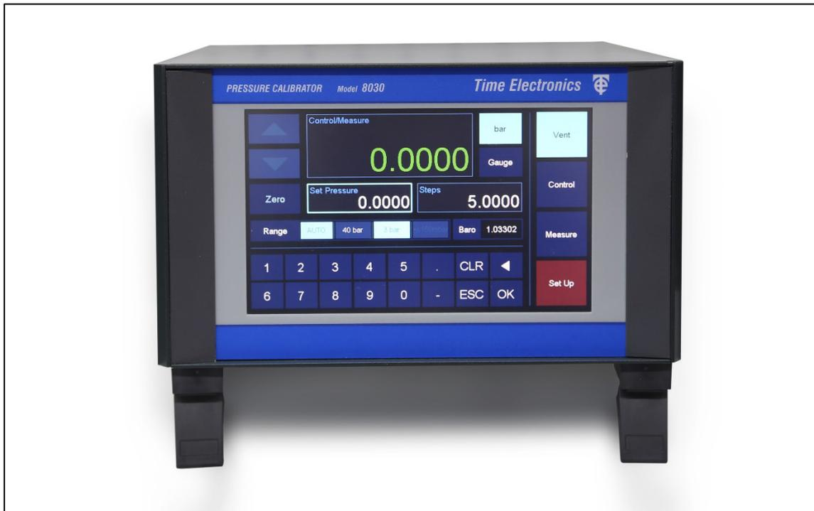
The front panel features a 7" TFT touchscreen, to display controls and instrument information.
