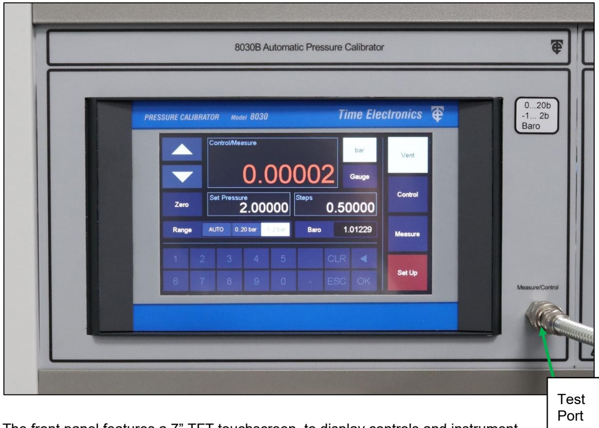
The front panel features a 7" TFT touchscreen, to display controls and instrument information. Additionally, the test port is accessed on the front of the console.
