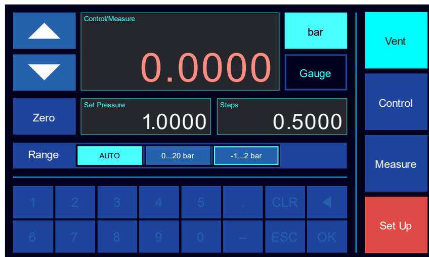
The pressure type selection button is only active if the controller is fitted with the barometric reference option (BARO).
