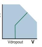
Some power sources, such as rechargeable batteries, can be damaged if their output voltage falls below a certain level. The 8029 provides automatic protection by incoprorating fully variable voltage dropout (CI, CR, CG and CP modes). If the voltage applied to the load falls below a preset level, the load current is rapidly reduced to zero.
