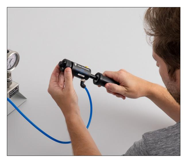
Pocket sized pumps that provide a simple and compact solution to field pressure generation. Each pump combines a smooth and controlled operation with a rugged yet lightweight design, making them the ideal tool for instrumentation engineers that perform site pressure testing.
