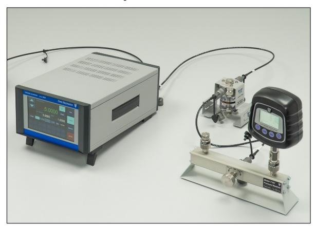
During transitions from a high pressure setpoint to a smaller one, liquid and residues present in the pneumatic system may flow into the 8030.
