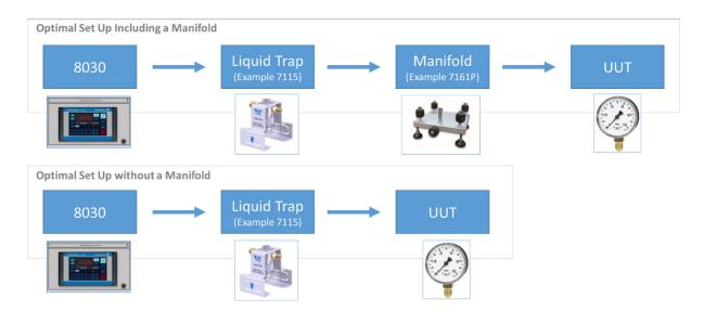
Minimess hoses are supplied for connection from the 8030 to the 7115. An additional hose is supplied for connection from the 7115 to the UUT. If an manifold is supplied this will be a minimess to minimess type. A minimess to ½ BSP or ½ NPT hoses will be supplied if required.
