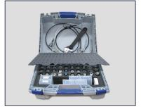
The 7198 pressure adaptor kit can also be used to make connections from the 7115 to various UUTs with different thread types.
