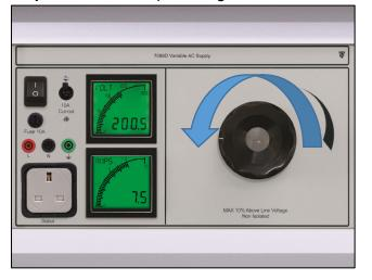
Step 3: Wind the output voltage control knob counter clockwise to zero the output.
