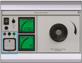
**Step 5:** Adjust the output voltage control knob clockwise to increase the AC voltage to the device.
