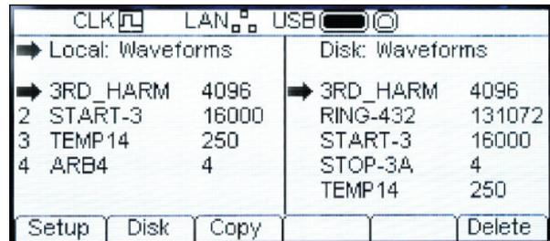
Both instruments incorporate a front mounted USB socket for connection of flash memory disk drives which can store up to 1,000 waveforms and 1,000 setups.
