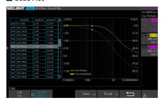
The 7024 can control the optional USB AWG module, scan a devices amplitude and phase frequency response, and display the data as a Bode Plot.
