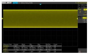
The 7024 can measure all sampled data points up to 14 Mpts. This ensures the accuracy of measurements while the math co-processor decreases measurement time and increases ease-of-use.
