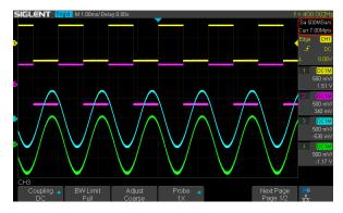
The oscilloscope has two 1 GSa/s ADC chips (channel 1 and 2 share one, channel 3 and 4 share another), so that each channel can achieve sample rates up to 500 MSa/s and work on bandwidths of 200 MHz when all channels are enabled.
