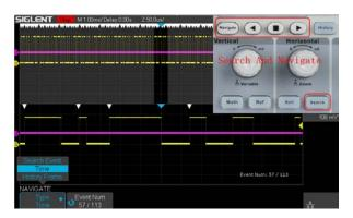
The 7024 can search events specified by the user in a frame. It can also navigate by time (delay position) and historical frames.
