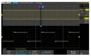
Through Gate and Zoom measurement, the user can specify an arbitrary interval of waveform data analysis and statistics. This helps avoid measurement errors that can be caused by invalid or extraneous data, greatly enhancing the measurements' validity and flexibility.
