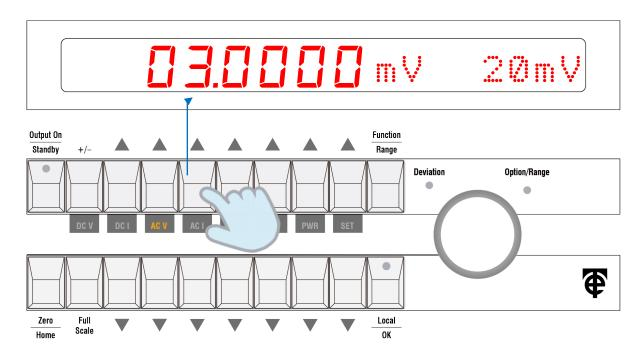
6. Output is initially disconnected from the output terminals. The LED on the Output On button flashes to indicate this. The LED beside the output terminals also flashes. Connect the signal to the output terminals by pressing the "Output On" button.
