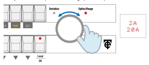
9. When the required current range is displayed, press the "**OK**" button.
