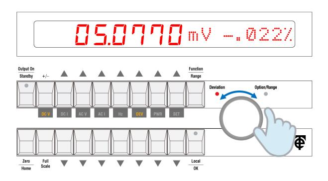
**Note:** It is not possible to adjust the deviation if the output setting is zero, since the deviation is a percentage of value. The deviation will be displayed as zero percent in this case.
