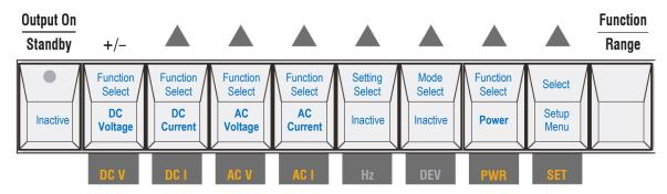
The **Function/Range** button can also be pressed after a function has been selected and is in use. The function indicators will flash show they are selectable.
