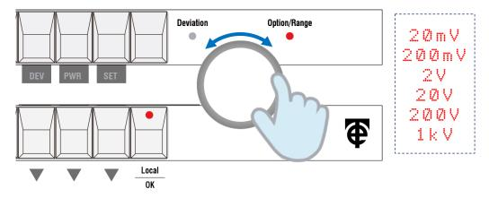
When the required range is displayed, press the "OK" button as highlighted by the flashing LED.
