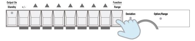
Now reselect the present function. For example, for DC volts, press the "**DC V**" button.
