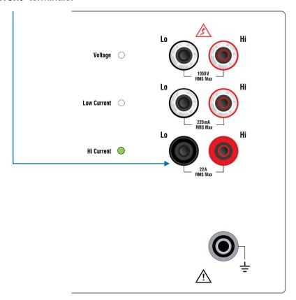
**Warning:** Currents in excess of 10A can be dangerous and leads with the correct current rating should be used. Do not leave high current switched for more than 20 Minutes.
