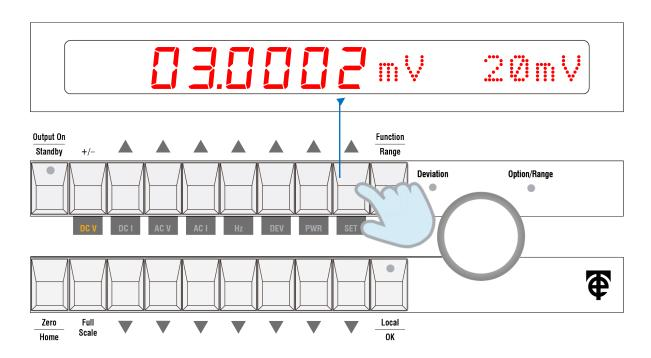
If necessary, the output can be turned off by pressing the "Standby" (output on) button.
