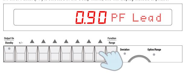
Use the "+/-" button to set either positive / negative phase or lead / lag PF.
