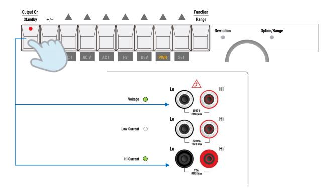
To change the output the previous steps must be taken to adjust voltage, current, phase and frequency. The 5077 will show and store the previous values for each of the settings.
