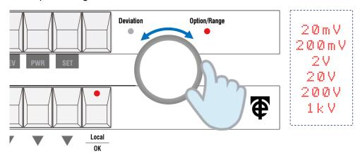
When the required range is displayed, press the "OK" button as highlighted by the flashing LED.
