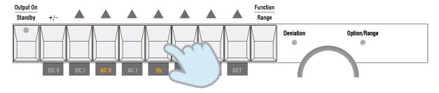
9. Then adjust the frequency using the "**Up** ( $\Delta$ ) / **Down** ( $\nabla$ )" buttons whilst the output is on.
