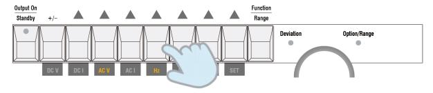
4. Select the frequency using the "**Up** ( $\Delta$ ) / **Down** ( $\nabla$ )" buttons.
