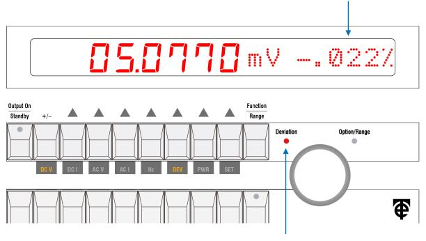
Deviation mode is highlighted by illumination of the "Deviation" LED. This prompts the use of the rotary knob.
