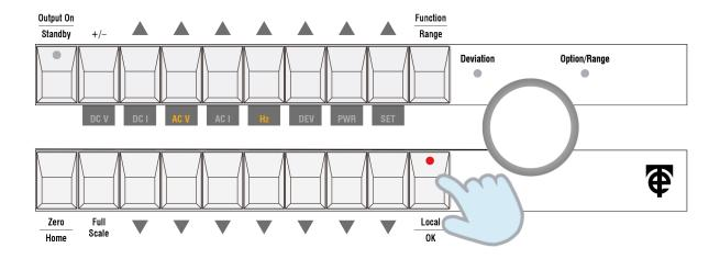
5. Once the frequency is set, the display readout will show the output voltage and operating range. The output value can be entered using the "**Up** ( $\Delta$ ) / **Down** ( $\nabla$ )" buttons.
