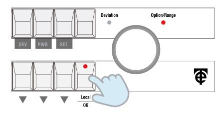
3. To set the required output voltage, increment or decrement the individual digits by using the "Up ( $\Delta$ ) or Down ( $\nabla$ )" buttons.
