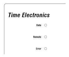
There are 3 LEDs located on the left-hand side of the unit's front panel.
