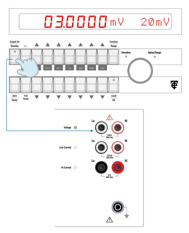
The Output button LED lights up constantly to indicate that the output terminals are live. The LED adjacent to the live output terminals also illuminates steadily.
