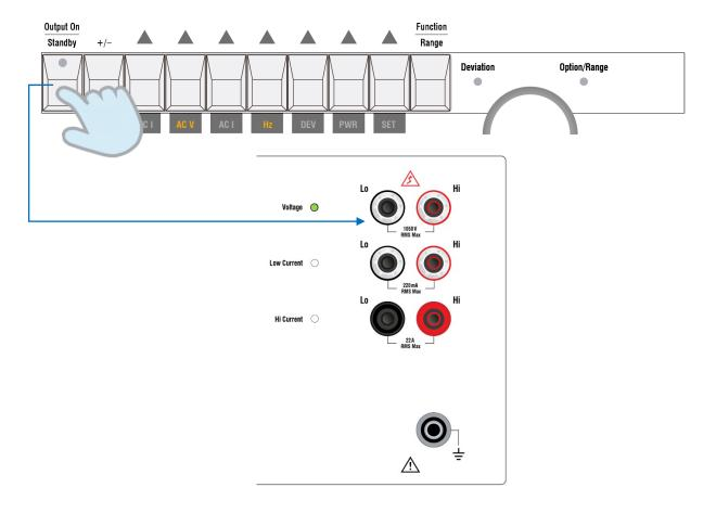
7. When the output is switched on, the operating range is no longer displayed and the set frequency is shown.
