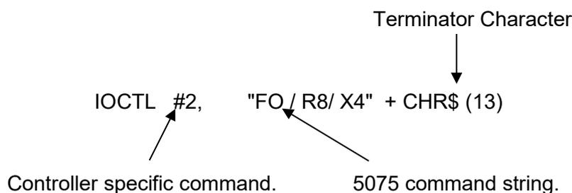
The controller specific command is an instruction to the IEEE controller to read or write the following string to the device on the bus. This command may vary considerably between controllers and the example shown is a typical QuickBasic language by Microsoft command. Refer to your IEEE controller for specific commands.
