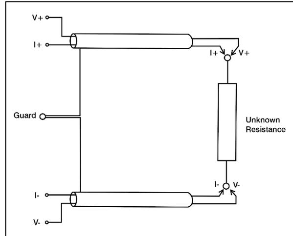
If high value resistances are being measured the guard may be taken to the casing of the resistor (if metal), or alternatively connected to a screen encasing the resistor. In most cases, grounding the resistor will make measurements noisier.
