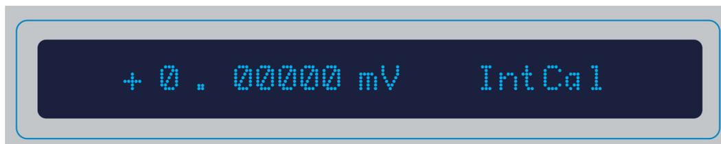
If this message is displayed on start-up, the 5075 will require recalibration. Refer to Re-Calibration in section 8 for further information. This may or may not disappear after a few seconds, depending on the options set in the user menu.
