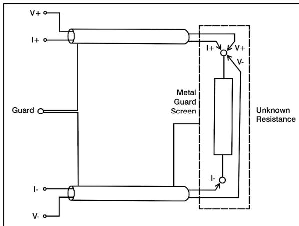
If making high value resistance measurements, the use of PTFE insulated cable would be an advantage because of its high insulation resistance.
