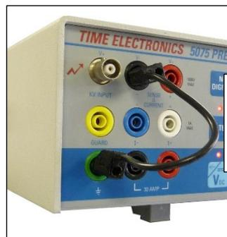
Using non-standard BNC lead V- Earth connection
