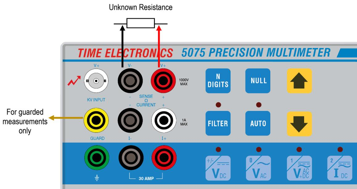
If the lead resistance is large in comparison to the value being measured, the readings will be inaccurate. Under these circumstances, the four terminal measurement method would give better readings however, the null function may be used to compensate for the lead resistance.
