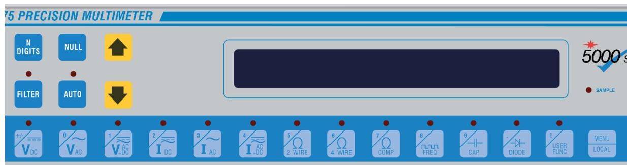
All the main functions such as range change or mode selection can be performed by one key-press.
