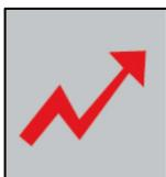
**The terminals marked with this symbol carry the potential of the source under test. These terminals and any other connections to the source could carry lethal high voltages and at no time should they be touched during a high voltage test. Switch off the source before attempting to rectify any problems associated with the test.**
