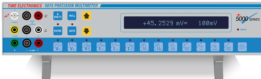
The 5075 is a benchtop digital multimeter combines high performance and accuracy with simple operation. With speed and precision, it measures from nanovolts to 10 kV, from picoamps to 30 Amps, from nano-ohms up to 1 G $\Omega$ , and from picofarads to 300  $\mu$ F. It is ideal for users requiring a cost-effective DMM with multiple functions and exceptional resolution and accuracy up to 7½ digits.
