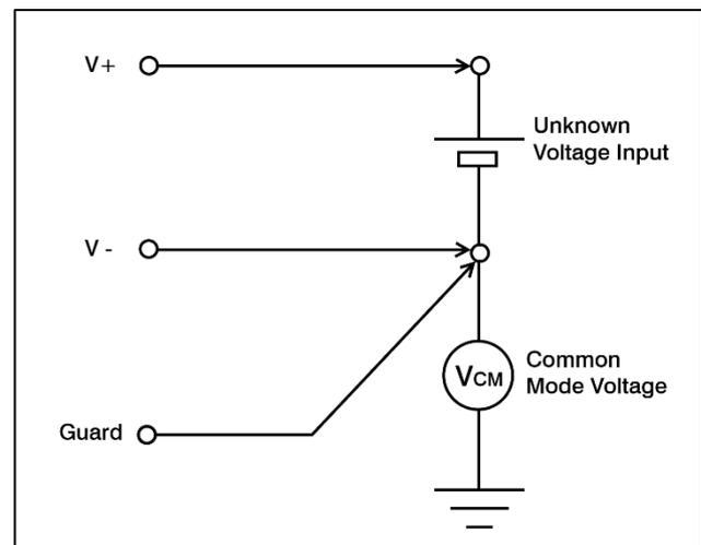
The use of the guard on AC measurements may still be applied as long as the source impedance is low enough not to be shunted by the extra capacitance introduced.
