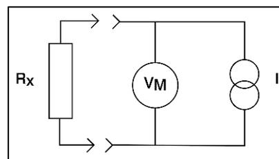
According to Ohms law, if resistor  $R_x$  was  $1\Omega$  and  $1A$  was passed through it,  $1V$  would be developed. If the value of  $R_x$  was higher, say  $1M\Omega$  and  $1A$  was passed through it by current source  $I$ ,  $1\text{Million Volts}$  would be developed across  $V_m$ ! (if the current source was capable of that voltage compliance).
