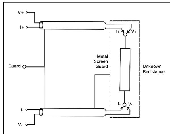
When making precision resistance measurements, ensure that the meter has been zeroed correctly. By following the connection diagram shown here, any induced EMF's and thermals are eliminated from the measurement.
