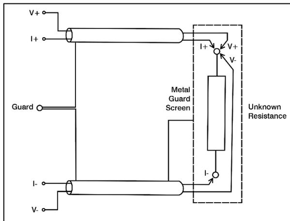
If making high value resistance measurements, the use of PTFE insulated cable would be an advantage because of its high insulation resistance.
