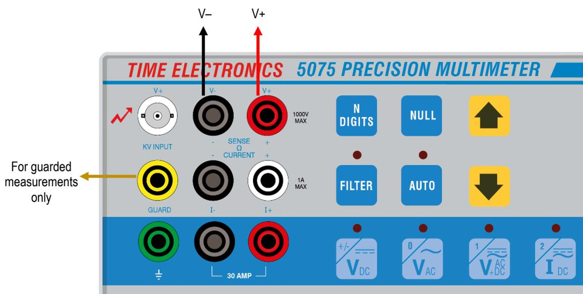
The disadvantage of this connection V+/V- method is that a loop is formed, and stray magnetic ac fields induce small voltages in the loop.
