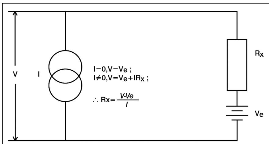
This method is only effective up to about 100 kΩ, but may be used on two or four wire ohms. The most effective solution is to not have thermals present in the first place.
