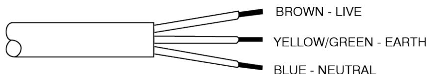
The wire colour coding may differ depending upon the lead supplied for the destination country. Normally an IEC approved molded wall plug will be supplied as part of the lead.
