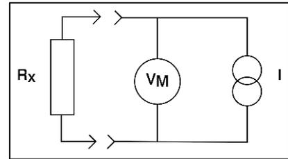
According to Ohms law, if resistor  $R_x$  was  $1\Omega$  and  $1A$  was passed through it,  $1V$  would be developed. If the value of  $R_x$  was higher, say  $1M\Omega$  and  $1A$  was passed through it by current source  $I$ ,  $1\text{Million Volts}$  would be developed across  $V_m$ ! (if the current source was capable of that voltage compliance).
