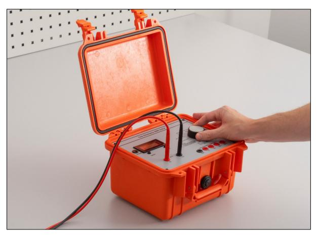
This 5068 provides all the equipment necessary to test and calibrate insulation test sets and megohm meters. It consists of:
