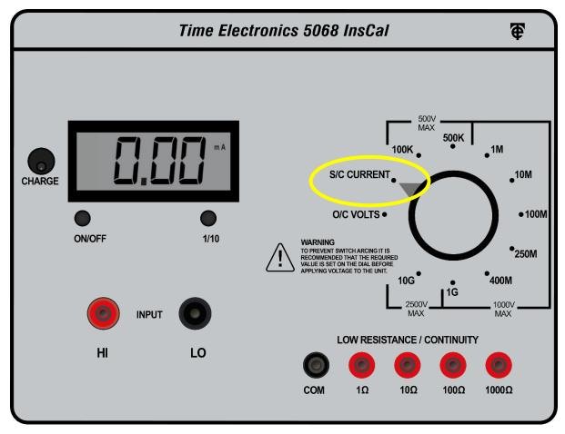
2) Using range selection button under the display, choose the required current range: 2 mA or 20 mA.
