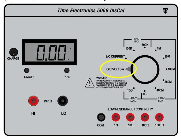
3) Using range selection button under the display, choose the required voltage range of 1.999 kV or 2.50 kV.
