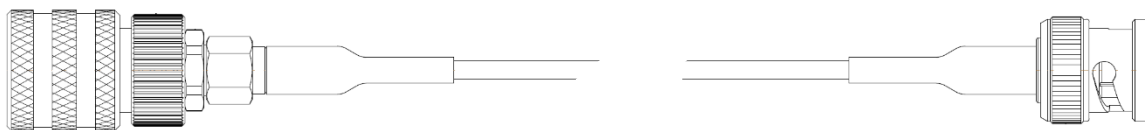
Quick Release SMA to BNC Test Lead (095-0069)
