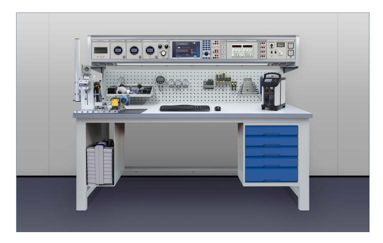
The CBP-TRN1 CalBench can be used to demonstrate and practice pressure, process, and temperature instrumentation calibration. It is suitable as a teacher workstation that is easy to operate manually, but can also perform software driven calibration. Educate trainees on applications relating to commissioning, calibration and maintenance of the typical devices used for measurement in industrial systems.
