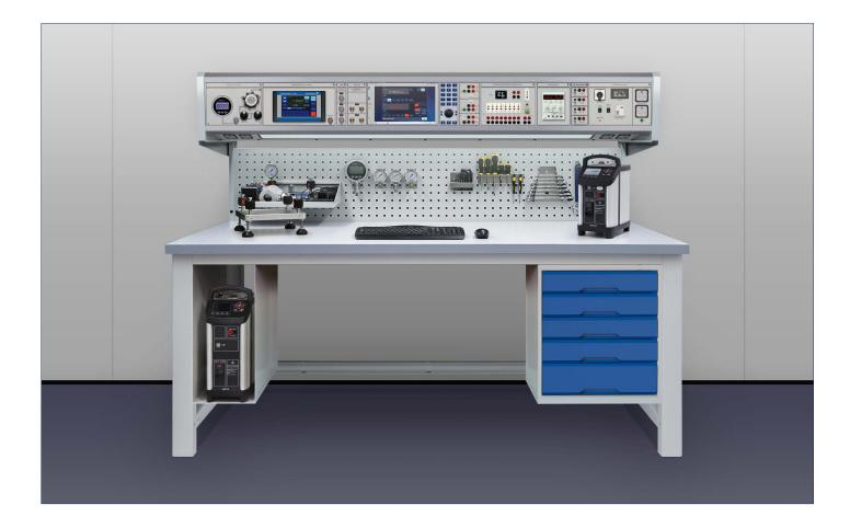
The CBP-PROC1 CalBench is a package that provides users with the capabilities to perform rapid calibration of process and pressure instrumentation. It is an ideal solution for instrument workshops that require a high performance workstation as the platform for calibration of plant devices and instruments.
