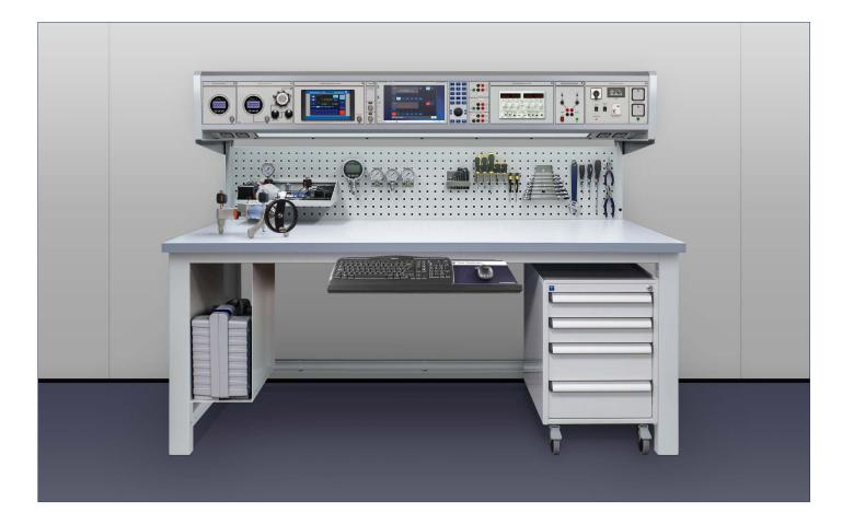
The CBP-PRES2 is a dedicated pressure calibration workstation with modules and extras that enable users to efficiently calibrate instrumentation like transmitters and gauges. It is an advanced system suitable for instrument workshops performing internal calibration and commissioning.
