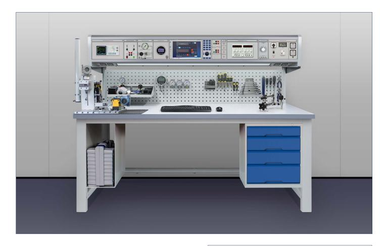
The CBP-TRN3 CalBench is a multi-parameter workstation for pressure, process, and temperature instrumentation calibration training. It features a selection of easy to use modules and extras for practicing instrumentation setup, connections and testing. Educate trainees on applications relating to commissioning, calibration and maintenance of the typical devices used for measurement in industrial systems.
