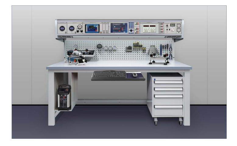
The CBP-PROC2 package is a high performance calibration workstation for testing and verifying process instrumentation. It has modules and extras to enable users to rapidly calibrate common pressure and temperature instruments such as transmitters, gauges, RTDs and thermocouples. It is an optimal solution for instrument workshops where users need to centralise their calibration and commissioning processes.
