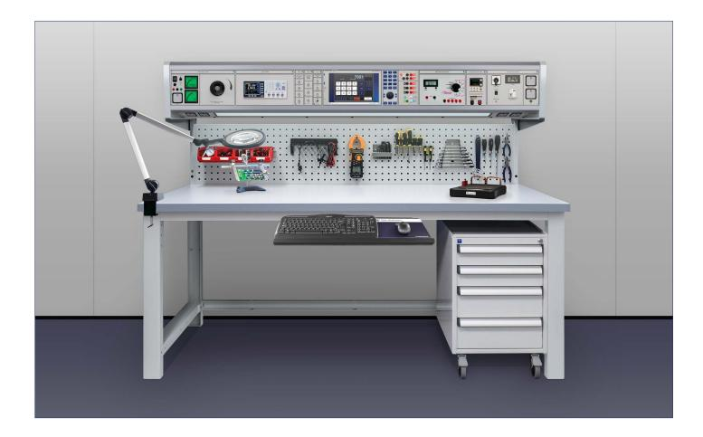
A CalBench package that provides users with a combination of modules and accompanying products for calibrating electrical and electronic test equipment and devices. It allows users to test and verify a wide range of instruments, with a high level of automation to ensure rapid turnarounds.
