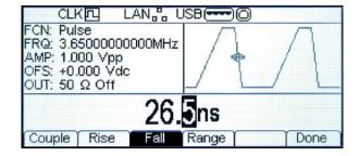
Both models incorporate a pulse generator mode which provides wide range pulse width and delay independent of period. Rise and fall times (edge speeds) are also fully variable.
