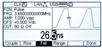
The 3.6" diagonal panel uses  $256 \times 112$  pixels and provides a large amount of simultaneous information. System connection information is shown on the top line. Below that is a general status screen showing five major parameters. These parameters change depending upon the function being used. Below the status information is the main editing line which shows the parameter currently under control.
