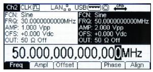
The generators are available in one channel or two channel versions, the latter incorporating two outputs with identical capabilities.
