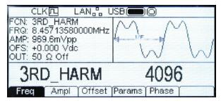
Both generators offer DDS generated arbitrary waveforms capability. A number of standard waveforms are included, and up to four user defined arbitrary waveforms can be stored in the instrument at any one time.
