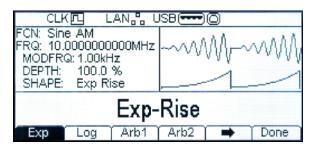
Both generators offer a comprehensive set of digitally based modulations. The internal modulation source can use any of the standard or arbitrary waveforms currently within the generator (including noise) thus removing the need for an external modulation source. A modulating frequency between 1 $\mu$ Hz and 20kHz can be specified. An external modulation input enables any external waveform source to be used when required. The external bandwidth is DC to 20kHz.
