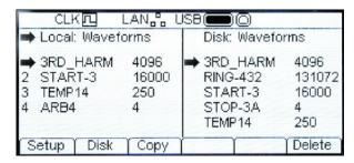
Both instruments incorporate a front mounted USB socket for connection of flash memory disk drives which can store up to 1,000 waveforms and 1,000 setups.
