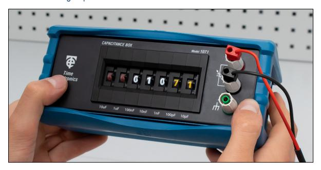
Before use it is recommended that all the digit thumbwheels are rotated completely 2 times. This will ensure the contacts are self-cleaned. This is particularly beneficial if the decade box has not been used for a long time.
