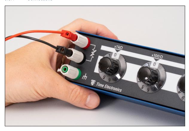
Connection to the decade box is via 4 mm safety terminal posts, using 4 mm shrouded or standard plugs. Alternatively, crocodile clips or stripped wire connections can be used.
