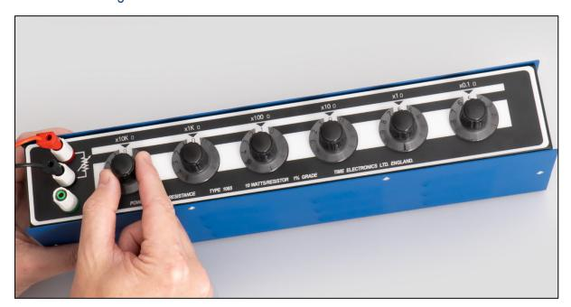
Switch contact resistance has been kept to a minimum by the use of multi-wafer switches, each with four parallel, silver plated, self-wiping contacts. Each range is scaled from 0 to 11, the maximum settable resistance is  $122,222.1 \Omega$ .
