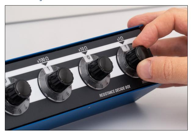
Use the front panel dials to set the required values according to the decade ranges. The selected value shown in the white setting window under the range arrow. This enables precise setting with a clear unambiguous indication.
