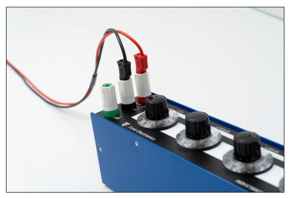
Connection to the decade box is via 4 mm safety terminal posts, using 4 mm shrouded or standard plugs. Alternatively, crocodile clips or stripped wire connections can be used.
