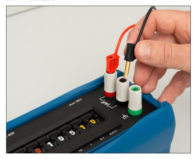
Connection to the decade box is via 4 mm safety terminal posts, using 4 mm shrouded or standard plugs. Alternatively, crocodile clips or stripped wire connections can be used.
