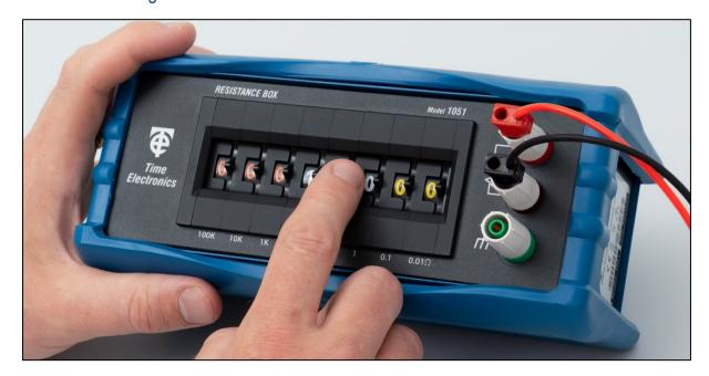
Before use it is recommended that all the thumbwheels are rotated completely 2 times. This will ensure the contacts are self-cleaned, maximizing their low contact resistance. This is particularly beneficial if the decade box has not been used for a long time.
