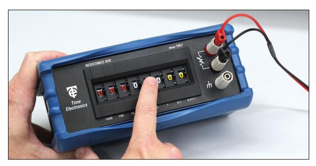
A precision resistance decade box designed for general laboratory work including platinum resistance thermometry. The 1051 is compact and durable, housed in a robust metal case with removable protective rubber cover, making it ideal for use in either the laboratory or field. Excellent accuracy is achieved by using high stability metal film resistors.
