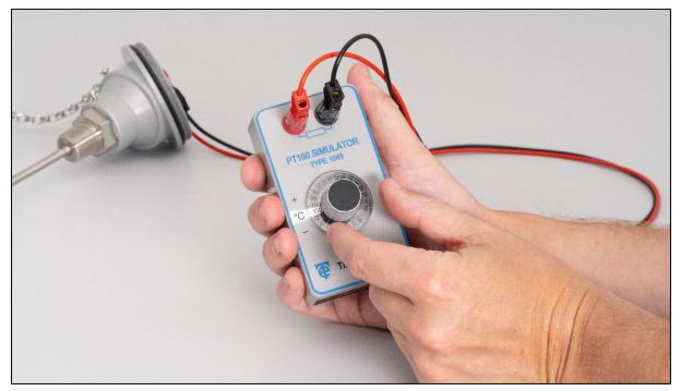
Connection to the 1049 is via 4mm standard plugs, or clamped bare twisted wires.
