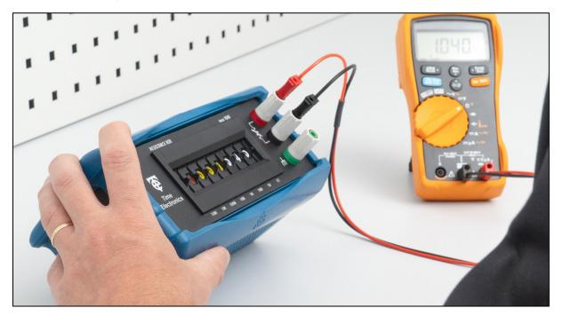
Before use it is recommended that all the thumbwheels are rotated completely 2 times. This will ensure the contacts are self-cleaned, maximizing their low contact resistance. This is particularly beneficial if the decade box has not been used for a long time.
