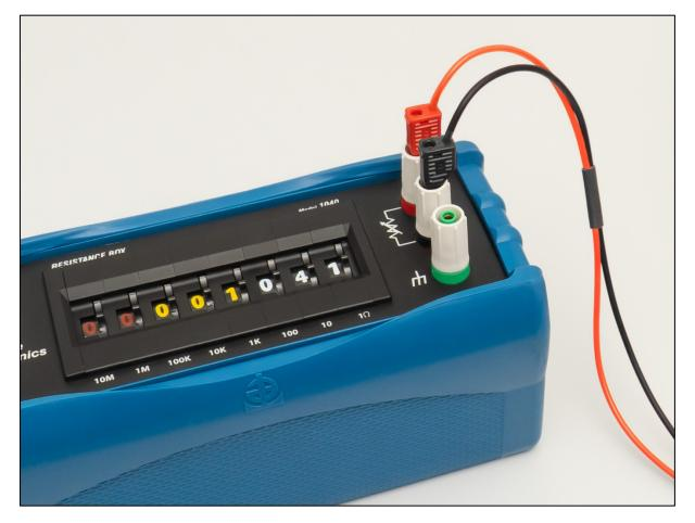
Connection to the decade box is via 4 mm safety terminal posts, using 4 mm shrouded or standard plugs. Alternatively, crocodile clips or stripped wire connections can be used.
