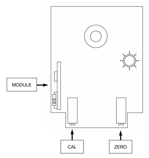
11. Turn the output adjustment pot. to full scale, and adjust the FS (CAL) calibration trimmer until the DVM reads 100 mV.
