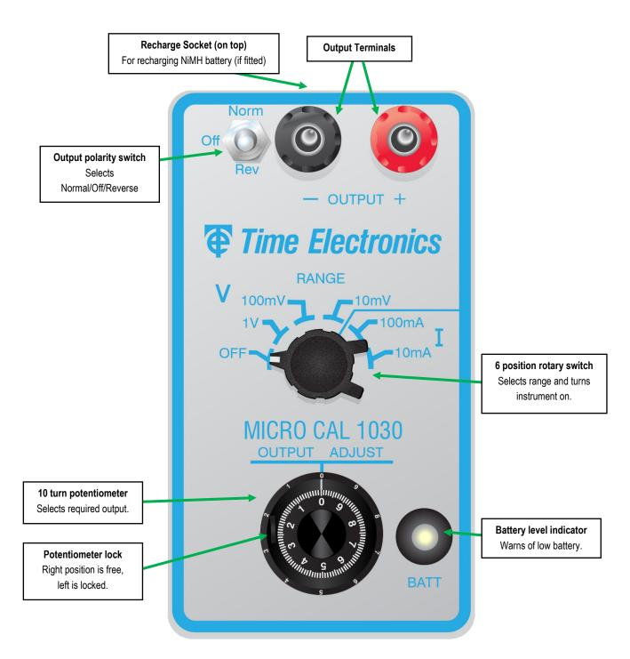
Note: Models built before March 2020 feature a different type of battery level indicator.
