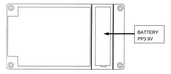
To recharge a NiMH battery, it is recommended that the instrument is turned off, in order to reduce charging time to the 15hrs minimum. The charger is then plugged into the recharge socket on the back. Note that it is NOT necessary to remove the battery to recharge it. The battery will not be overcharged if the recharger is connected continuously.
